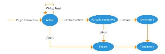
In transaction execution the circles mean state of the operation, and the arrows are the operation it self.
